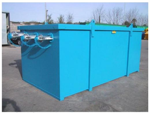
Figure 3.2f Example of Temporary Sediment Settlement Tank
