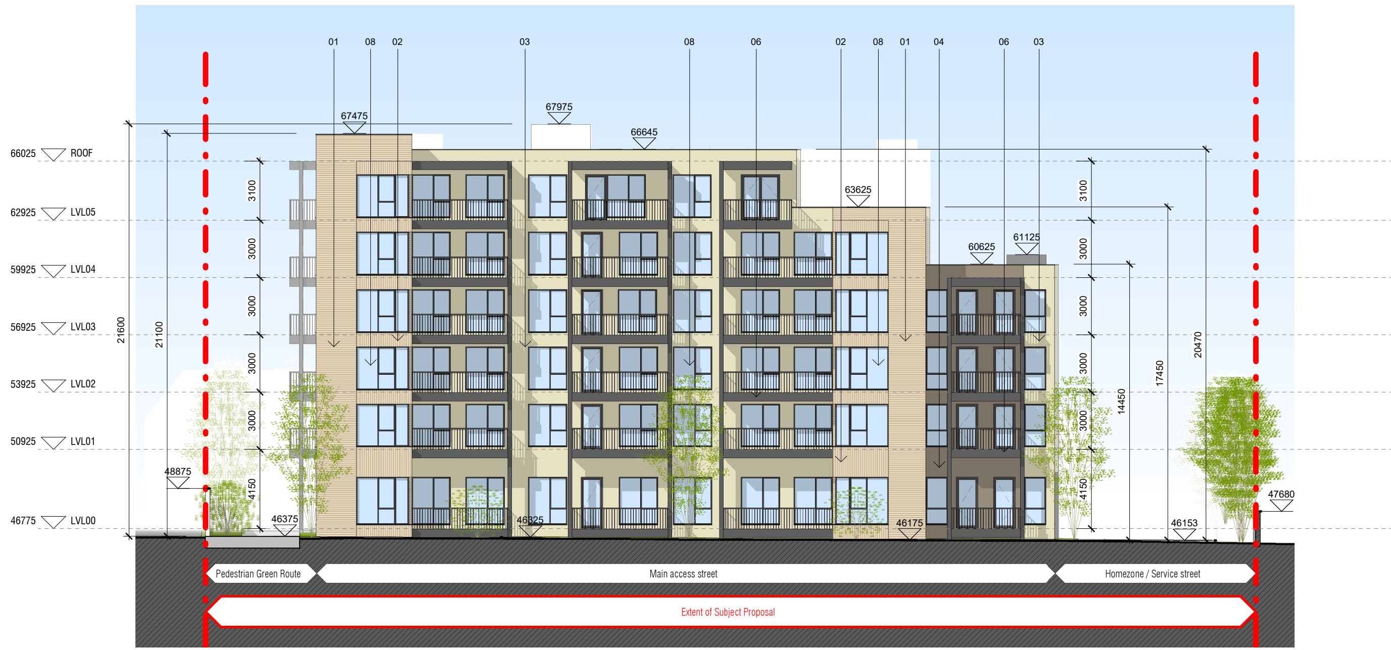
1 Site Elevations - Block3 East Elevation 1 : 200
